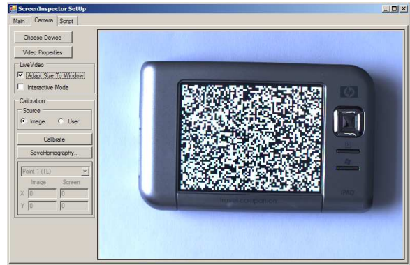
Fig. 4: System setup and calibration GUI, with an example of suitable calibration pattern
