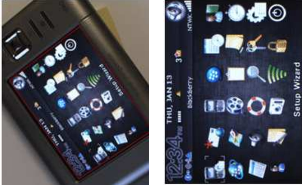
Fig. 5: Projection matrix estimation and screen image rectification (left: detected screen area, right: rectified image)
