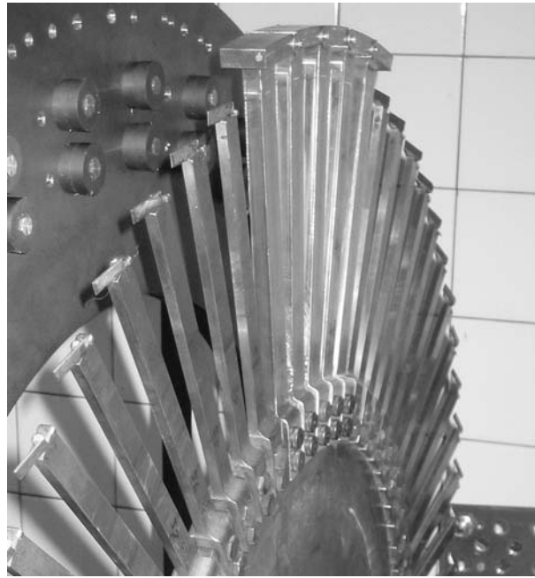
Fig. 4. Blade packet with friction elements
