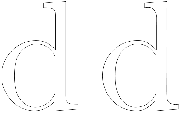
Figure 5: Two piecewise cubic Bézier curves describing the outline of the character "d" - 24 cubic segments (left); the corresponding piecewise interpolatory subdivision curves - 9 single-piece subdivision curves, 33 points, 24 tension parameters (right).
