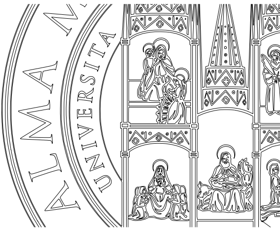
Figure 7: Outline of a detail of the University of Bologna logo: 561 piecewise cubic Bézier curves - 6679 cubic segments (left); reconstruction via interpolatory subdivision curves with local control - 561 single-piece subdivision curves, 7240 points, 6679 tension parameters (right).
