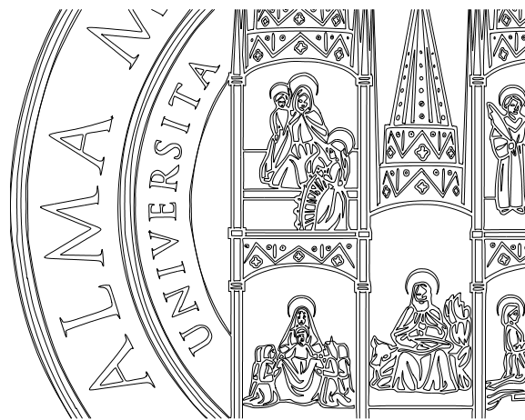
Figure 7: Outline of a detail of the University of Bologna logo: 561 piecewise cubic Bézier curves - 6679 cubic segments (left); reconstruction via interpolatory subdivision curves with local control - 561 single-piece subdivision curves, 7240 points, 6679 tension parameters (right).
