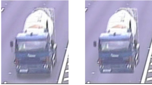
Figure 11: Left: synthesized vehicle using a shadow map. Right: synthesized vehicle without using a shadow map.
