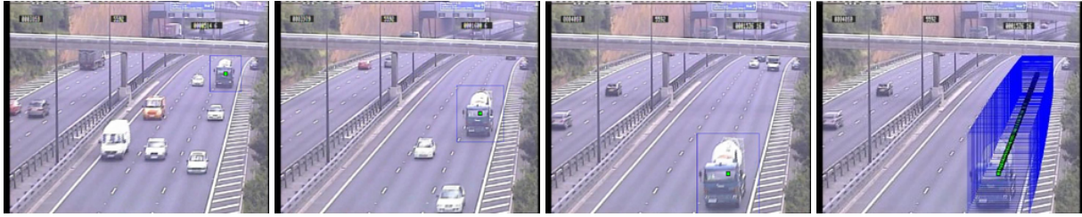
Figure 2: Windows drawn around a particular vehicle by the user, with on the right a calculated trajectory for the vehicle.
