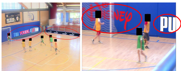
Figure 13: Virtual advertising example. Virtual billboards (highlighted by the red ellipses) are positioned in the scene using a chroma-keying technique.
