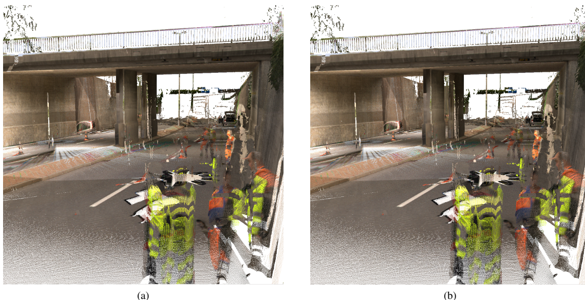
Figure 4: Comparison of (a) OpenGL rendering and (b) OpenCL rendering. As one can see, rendering results are almost identical. There are only small differences in far away parts of the scene, because we use eight bits more depth buffer precision than OpenGL. While the OpenGL version runs at about 5 frames per second, our implementation reaches 56 fps.
