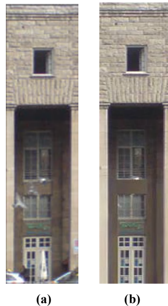
Figure4: (a) is a vertical slice texture which is cropped and rectified from the perpendicular picture of the facade and (b) is the same texture after removing the disturbing objects (e.g. flying birds, moving cars and moving pedestrians and so on). To reduce the complexity, the inside geometries were neglected as well.
