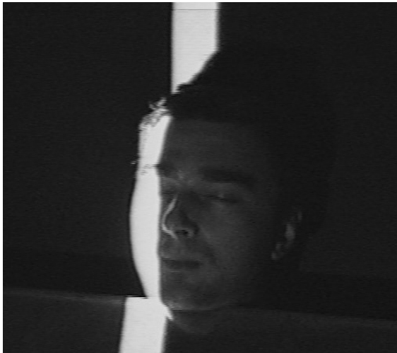
Figure 2. Human face while scanned by hard edge stripe; image captured by camera2
