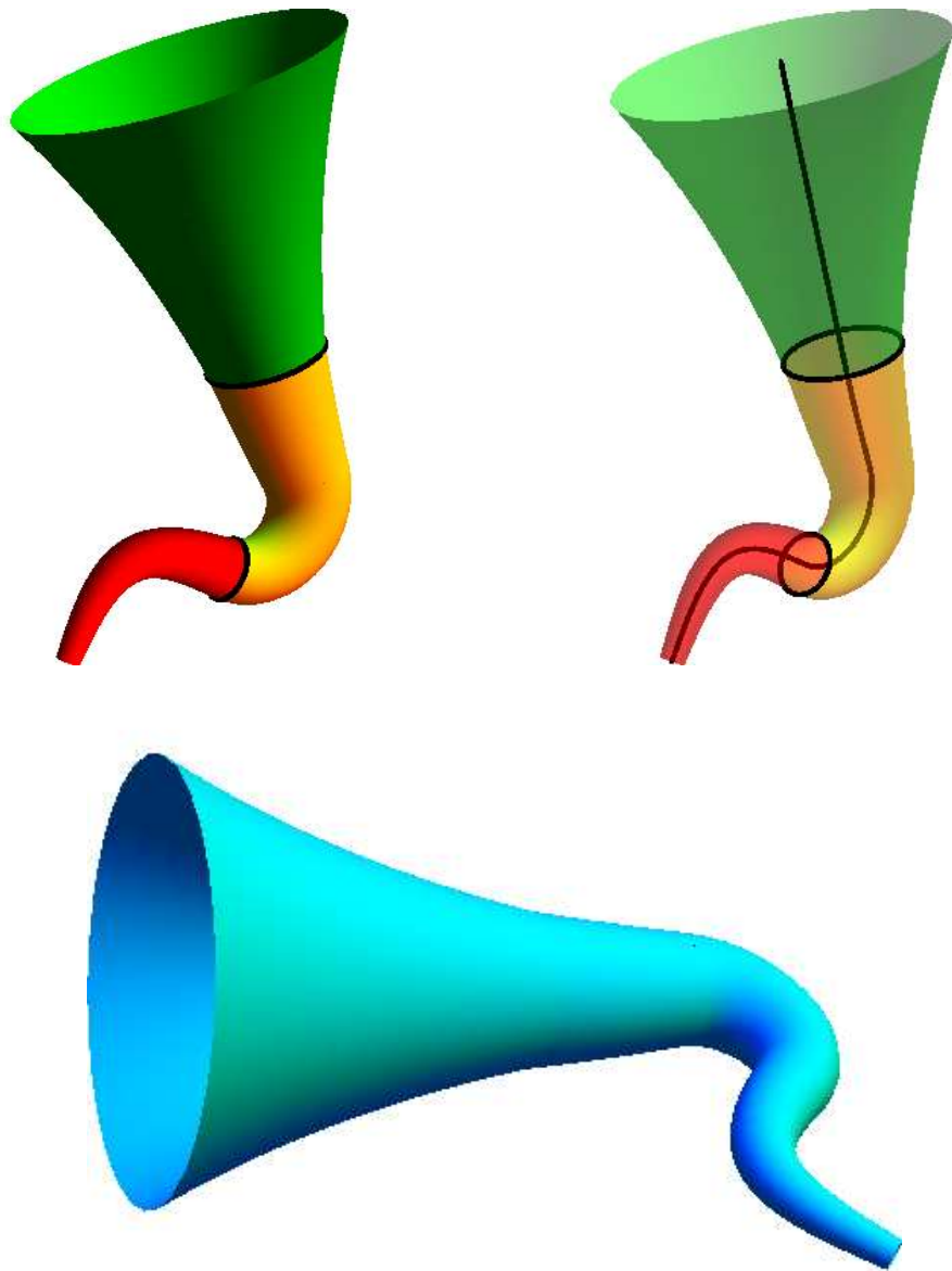
Figure 6.9: Two canal surfaces joined by a canal surface with biarc spine. Red canal surface is defined by (6.35). Green canal surface is defined by (6.36). Joining canal surface with biarc spine is shown in yellow.
